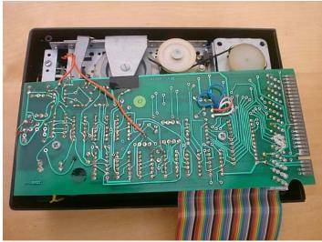
A componet view (sort of) of the above PCB. The large chip is the ROM, a N82S141N, which is a 512 byte PROM. The only analog chip I've seen in the PCB is a TL082 (dual op-amp). There is a CD4007, which I think sits between the analog and the digital part, as it has three CMOS inverters that can be externally wired to obtain NOT gates, NOR gates, NAND gates, etc, so it may be needed to square shape the signal amplified in the TL082.
