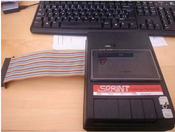
The Sprint continues the rear bus, so joystick interfaces and the like are possible. The unit has the "disable switch" (a 5 GBP add-on at the time) that let the user to disable the Sprint ROM without having to turn the computer off, remove the ribbon cable, then turn on.
